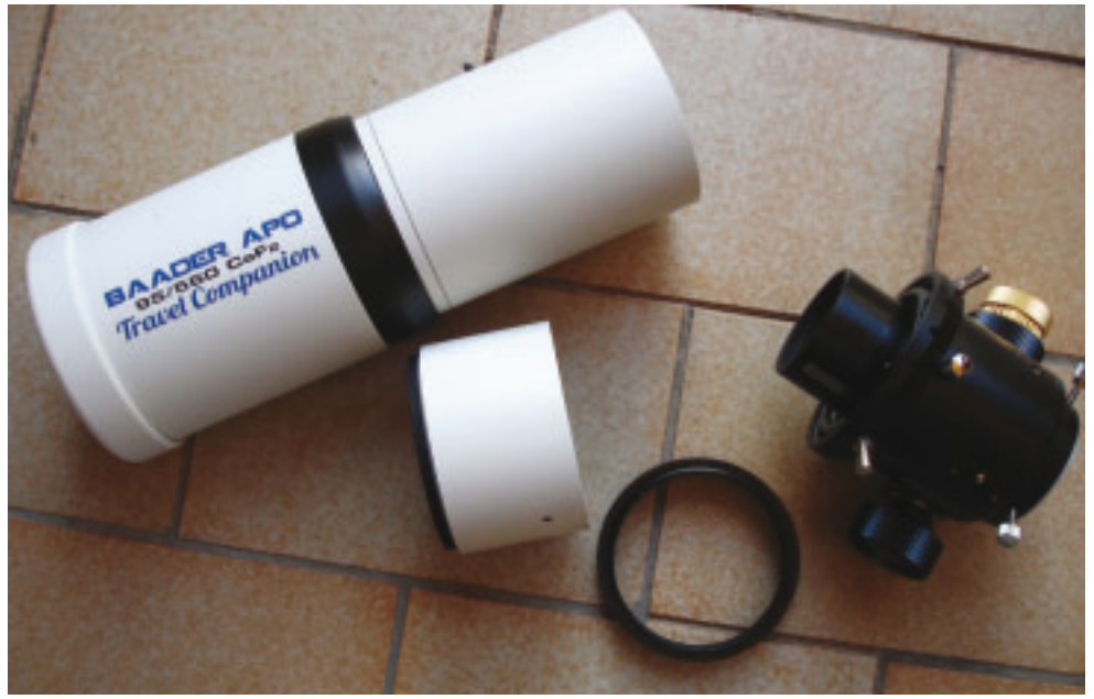
Image 3 - Disassembling the scope reveals a 60-mm-long tube extension.
