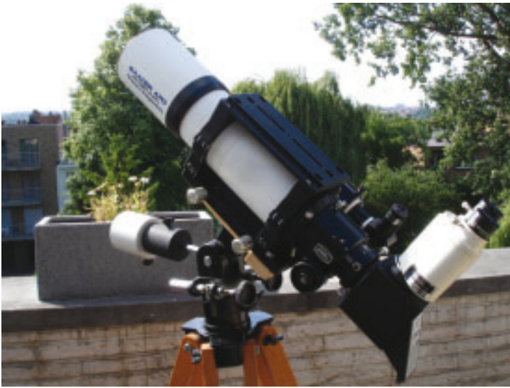
Image 4 - By unscrewing a 60-mm-long extension tube, the tube length is reduced to only 395 mm, allowing use of a binoviewer or a Herschel wedge without the need of additional transfer lenses.
