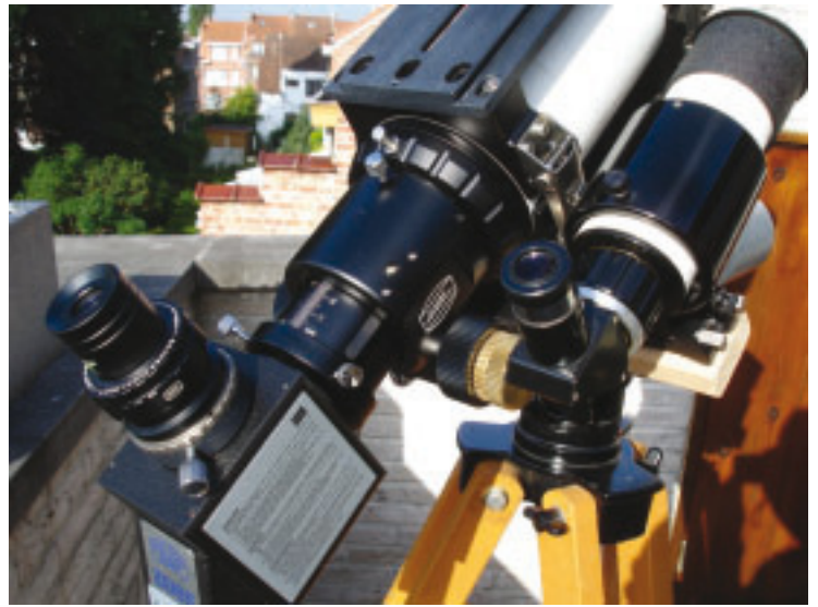
Image 5 - The Steeltrack focuser is a black-anodized 50.8-mm (2.0-inch) Crayford type. The right knob has a 1:10 precision reduction gearing. The drawtube travel is 75 mm and the focuser features a scale graduated in millimeters and inches.
